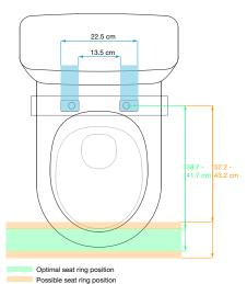
Left to right movement range of 4.5 cm Hole spacing tolerance of 9 cm
